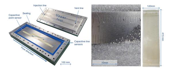
Figure 2: The 1D-CapaVisco system used for the RTM-oriented viscosity measurement (left), micro-glass spheres as positioned in cavity before (middle) and after infiltration (right).
