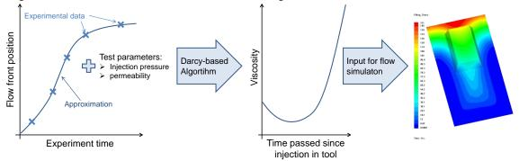
Figure 1: Calculation of the time-dependent viscosity of resin injected in to the tool based on the experimental data and possible usage of result for LCM simulation.
